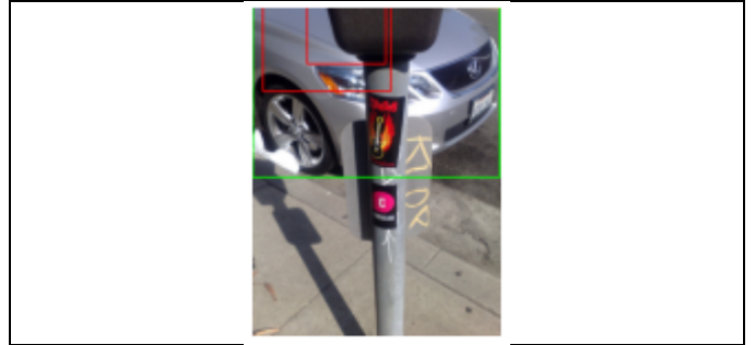
Figure 2.4.3: An example of false positives produced by SSD (correctly identifying a car, but the predicted bounding boxes are under the IoU threshold in relation to the ground truth box)
