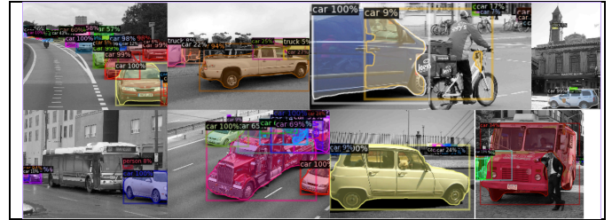
2.2.4: Examples of predicted bounding boxes and masks from COCO validation set, fine-tuned Mask RCNN on the COCO car subset
